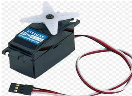
The PWM sent to the motor determines position of the shaft, and based on the duration of the pulse sent via the control wire the rotor will turn to the desired position. In this project the servo motor returns around 90 degree for opening the door and there is a switch will control the servo motor when it closes.
