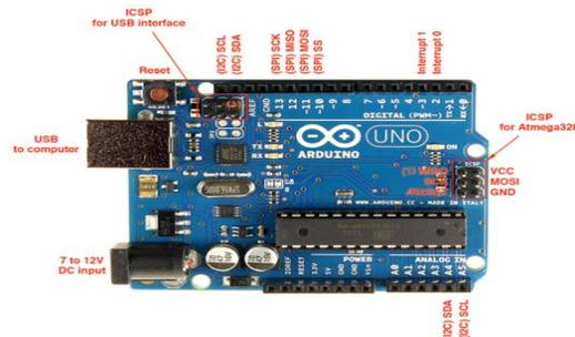
The Uno differs from all preceding boards in that it does not use the FTDI USB-to-serial driver chip. Instead, it features the Atmega16U2 (Atmega8U2 up to version R2) programmed as a USB to-serial converter.
