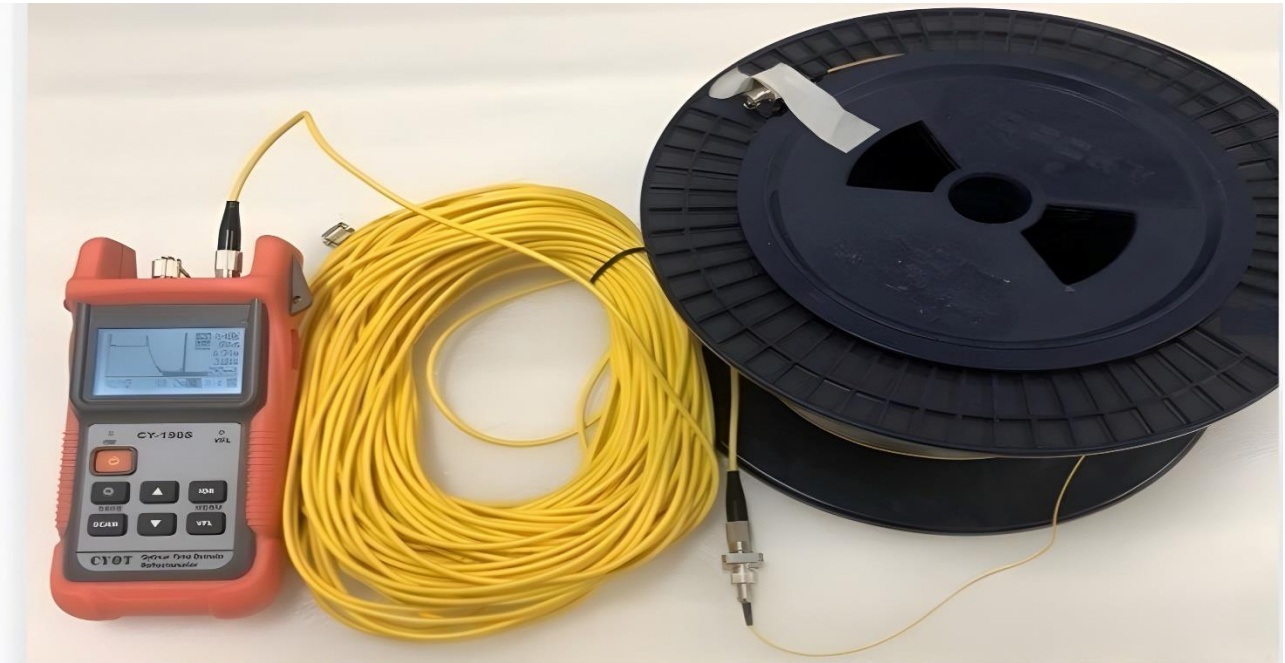
Figure 3.2: OTDR Testing a Fiber Spool
